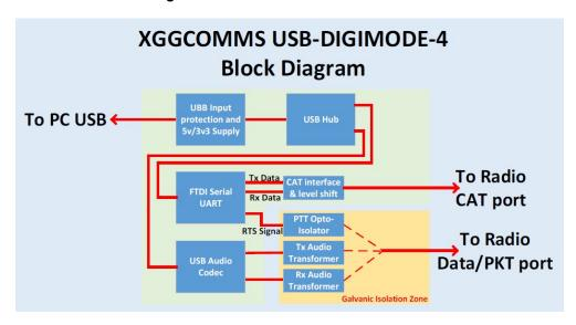
Internally, the interface utilizes the highly reliable FT232R USB UART IC to provide CAT & PTT control and the C-Media CM108 audio codec for the Tx/Rx audio interfacing. As both the FT232R and CM108 require their own USB connection, the interface has an internal USB Hub at the front end to provide the single USB connection to your PC.
